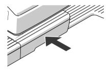
Slide the drawer in to the stop. Make sure that the drawer latches correctly on both sides.
