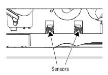
The sensors in the letter receiving wall are now accessible from the front (operator side).
