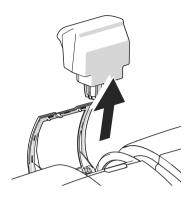
• Remove sealant tank out of housing.
