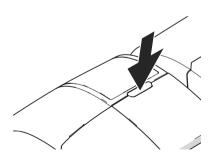
The sealant tank is located under the transparent flap. To open the flap:
