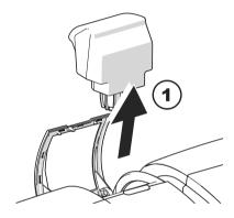
• Remove sealant tank out of the housing and put it at a safe place.
