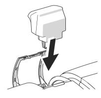
• Insert sealant tank into the housing with the cover downward.
