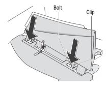
Hold sealer in place, and exerting moderate pressure, push the rocker onto the sealer such that the two clips engage on the bolts.
