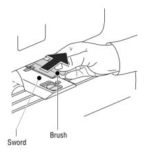
The brush is provided with pins on both sides that are snapped in clips on the sword.
