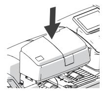
• Push the roller transport down powerfully until it locks into place.
