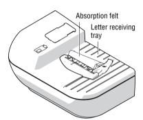
Bend the upper part of the felt to the right and push it beneath the letter receiving tray until it reaches the stop in the contour.
