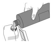
• Fill the sealant tank with SEALIT sealing fluid.
