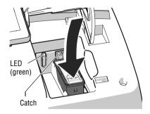
Slightly push the cartridge down on the "Push here ..." mark. In doing so, the cartridge tilts to the front.
