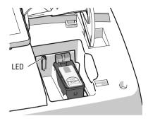
When the cartridge is inserted correctly, the green LED glows continuously.
