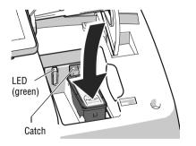
Slightly push the cartridge down on the "Push here ..." mark. In doing so, the cartridge tilts to the front.
