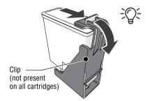
Note: Depending on the model, the ink cartridge may be fitted with a clip that acts as a transportation protection.
