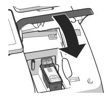
· Close the flap of the print system: Push down the flap in the area of the PostBase Vision logo until the latch catches.
