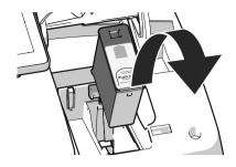
Take the ink cartridge upward and out of the socket.
