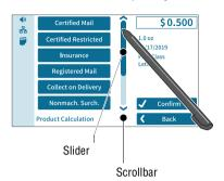
Press the slider and move it in the desired direction.
