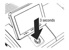
Press the ON/OFF button for three seconds to turn the PostBase Vision off.
