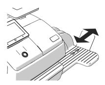
The catch tray can be adapted to different envelope sizes (up to 10" × 14") by displacing the catch bracket.
