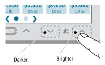
Press and hold the desired function (brighter / darker) until the display shows the desired setting.
