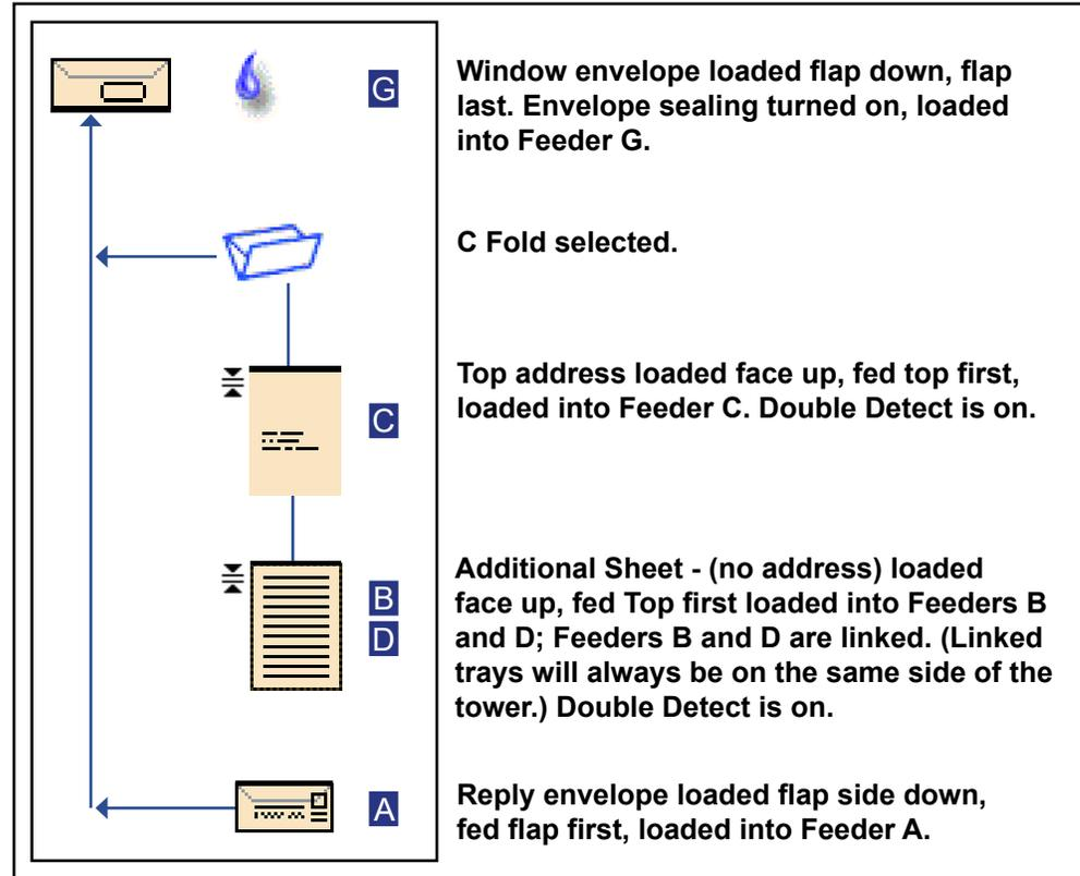
\* In the example above, the top address, additional sheet and C fold icons represent a set. That is, the Top Address and Additional Sheets are accumulated together, into a collation and the C Fold is applied to the collation.
